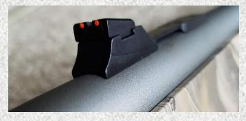
...or, I could add material to the front sight. I decided on the latter in the form of shims. That would allow me to confirm the proof of concept, preserve the sight's original design and integrity, and protect my warranty until T/C responded with a better solution.
