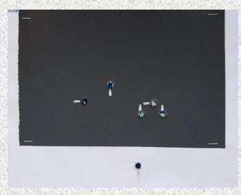
The six shims changed my average POI at 100 yards from 7" high to 2.5" high. That meant each shim, on average, brought down the POI 0.75". I estimated I would need ten more shims to bring the POI down enough for me to move the rear sight closer to the middle of its adjustable range.
