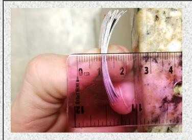
Below is picture of all of the shims stacked on top of one another ready to be installed.
